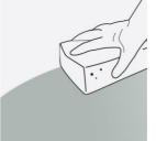
Sponge up and extract released residues. Go over 2 further times with clean water. Change rinsing water frequently.
