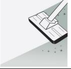
STEP 3. Add a little water and gently scrub surfaces with a white pad to release the loosened matter from the surface.
