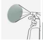
STEP 1. Spray a small amount of cleaner onto the surface.
