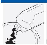
Dilute solution 1:10 with cool water. Mask and protect areas not to be cleaned
