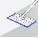
STEP 2. Spread out evenly and thinly using a sealant applicator pad.
