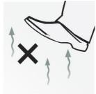
STEP 5. Newly sealed and finished surfaces should be left to dry for a minimum of 12 hours before allowing traffic.
